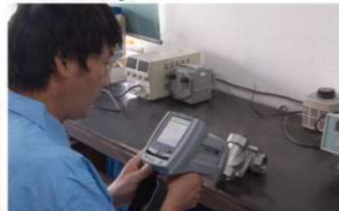
▲ German OXFORD X-MET5000 Spectrometer All the metal components of solenoid valve have been tested by OXFORD spectrometer to ensure the rightness of material, which meets various requests for production.
