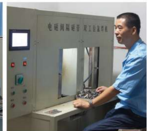
▲ Digital Automatic TIG Welding Machine Each plunge tube is processed by automatic welding machine, to ensure the product tensile strength and air capacity, further improve the welding quality.
