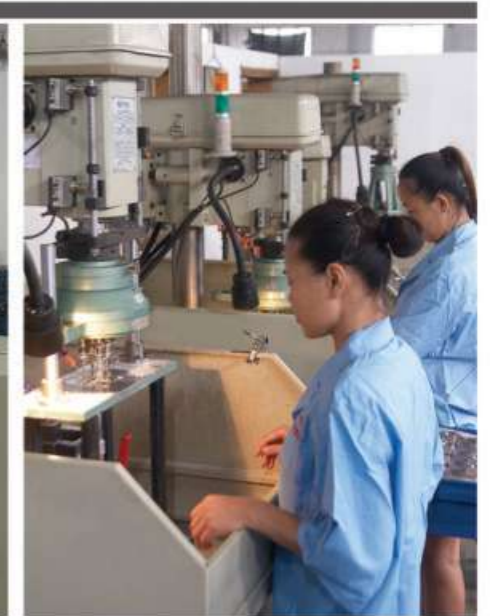
▲ High Precision Automatic Holes Drilling Machine The hole of valve cover is positioned and drilled at one time, to ensure the precision, and improves the production efficiency.
