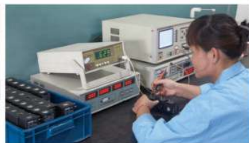
▲ Performance Testing Machine For Solenoid Coil To guarantee the quality, each solenoid coil has been tested in the aspects of resistor, laps, current, power and withstand voltage.
