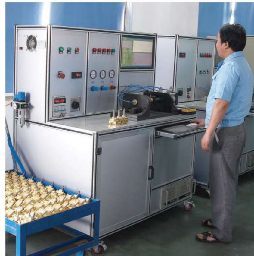
▲ High Performance Digital Automatic Testing Machine For Solenoid Valve Each solenoid valve has been tested of high pressure, low pressure, leakage and so on, to ensure that we can offer satisfied products for our customers.
