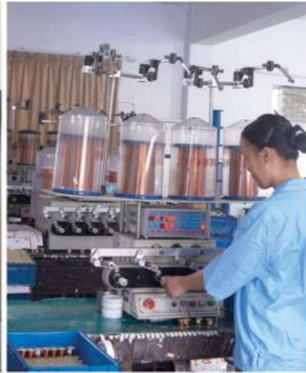
▲ Automatic Digital Winding Machine For The Production Of Coil We use automatic digital high-speed winding machine for the production of coil. The machine is characteristic of parallel winding, high precision and high speed.
